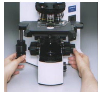
U-SVLB-4 mechanical stage with left-hand control & tactile covers
